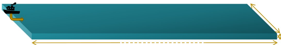
Figure 5. Schematic figure showing the vessel, the discharge and the ship wake formed behind the vessel. The figure is not to scale for practical reasons but is included to illustrate the simplified shape that the ship wake is assumed to take with constant depth and width.
